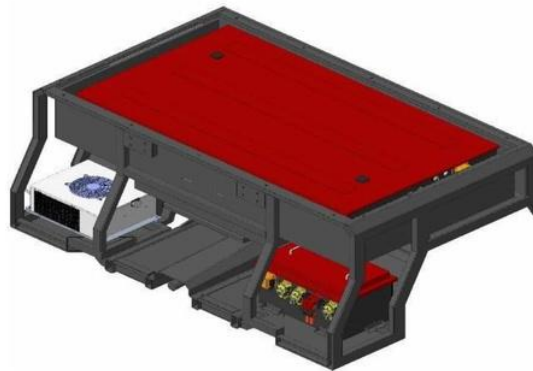
Fig 1. Battery System: Battery pack with PDU and BTMS mounted inside vehicle's frame
